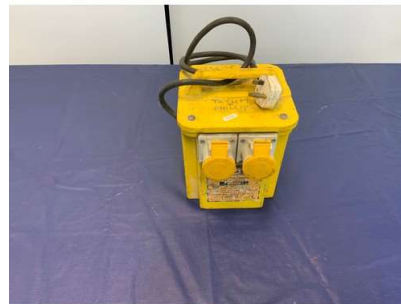
111. M - 3.3KVA 110V TRANSFORMER
