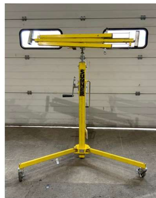
160. V - PLASTER BOARD LIFTER
