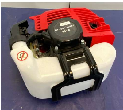
141. M - 52cc 2-STROKE PETROL ENGINE FOR A BRUSH CUTTER
