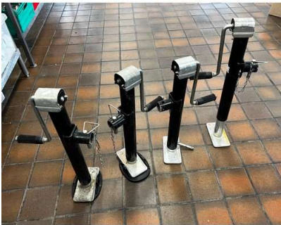
10. V - 4 x Jack - 580-970mm H/Duty Side-Wind T/Scopic Swivel Jack RRP £55 EACH - USED FOR STEADYING, LEVELING, AND SUPPORTING UTILITY, PLANT, OR TRAILER BEDS
